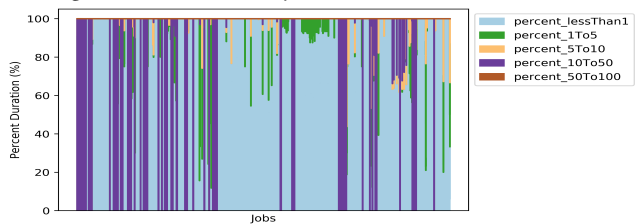
Figure 5: % I/O duration vs. write burst size as % of memory.
